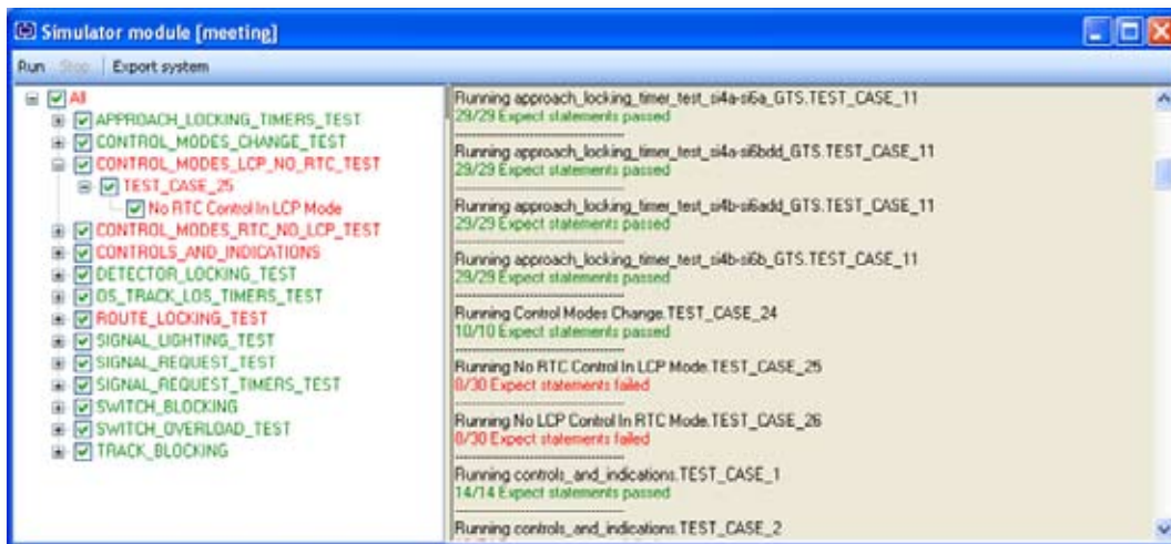
Figure 5. Prover iLock Simulator runs through all test cases, marking passed tests green, and failing tests red.
